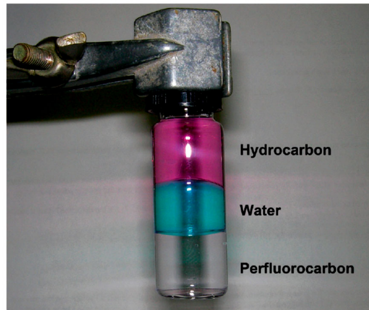
Fig. 1 A triphasic system as an example of the immiscibility of PFC solvents with both aqueous and organic phases.
