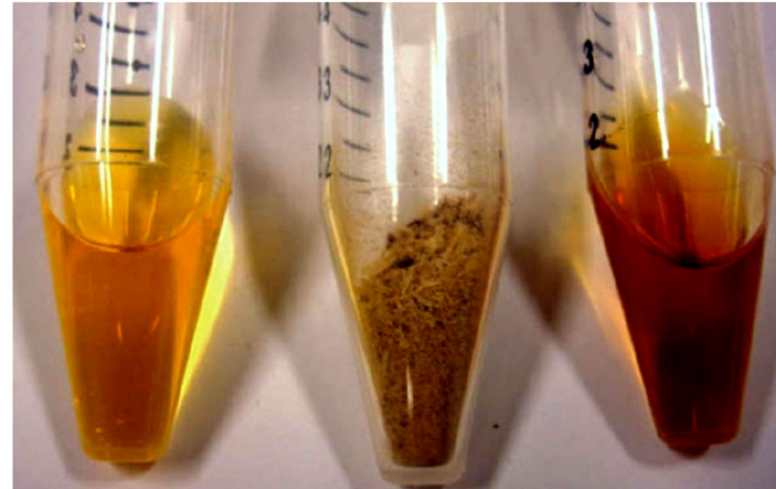
Fig. 20 Dissolution of beech powder in [\text{C}_2\text{C}_1\text{im}][\text{MeCO}_2] ; left: ionic liquid, middle: beech powder, right: solution. Reproduced from ref. 114.
